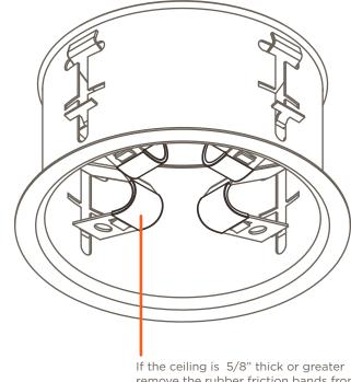
If the ceiling is 5/8" thick or greater remove the rubber friction bands from the springs.
